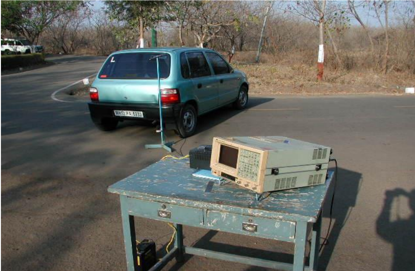
Fig. 2: Stationary Noise Measurement Set-up
