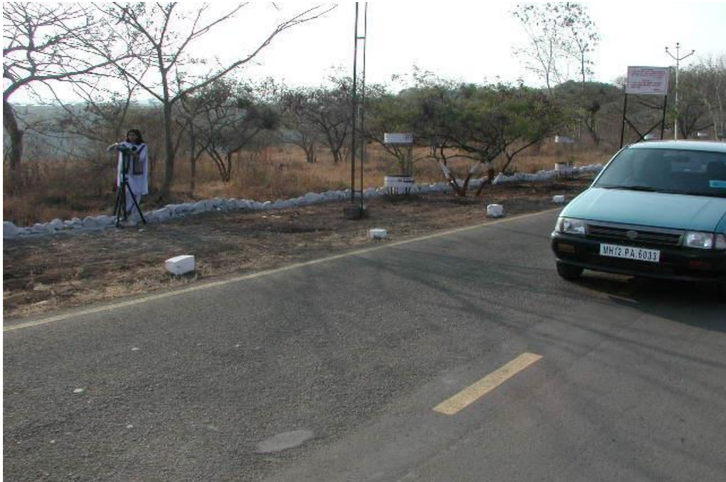
Fig. 1: Pass-by Noise Measurement Set-up
